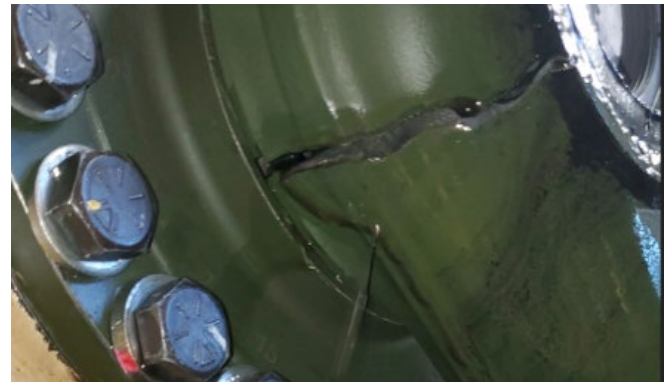
Figure 11: Prototype Spline Burst
