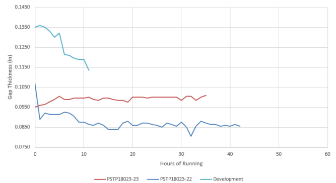
Figure 12: Thrust Washer Wear
