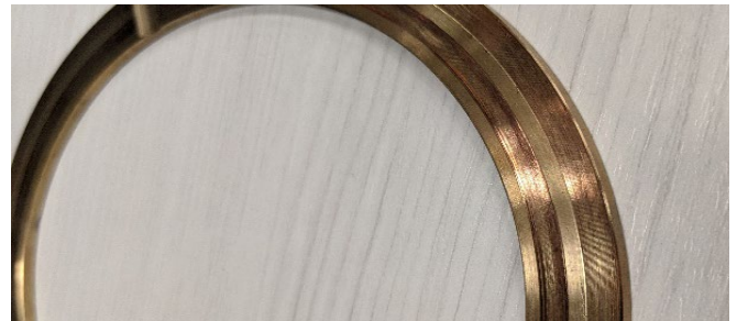
Figure 13: Thrust Washer Wear Patterns
